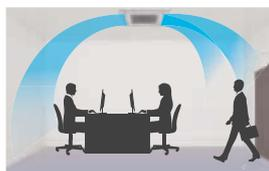
Comfortable air conditioning by preventing direct blowing of cold air and by providing swinging air flow simultaneously.
